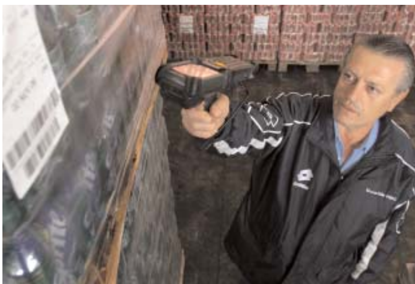
A traceability system for product pallets has been developed and installed in all Coca-Cola HBC production plants, warehouses and depots within the European Union. The system uses a label with unique production information and wireless scanning guns.
