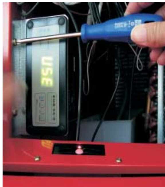
Energy saving devices for cooling equipment like this EMS-55 unit record events such as passing consumer traffic, door opening frequency and store downtime then adjust compressor and light usage accordingly. From 1 January 2007, these devices are being installed in refrigeration equipment.
